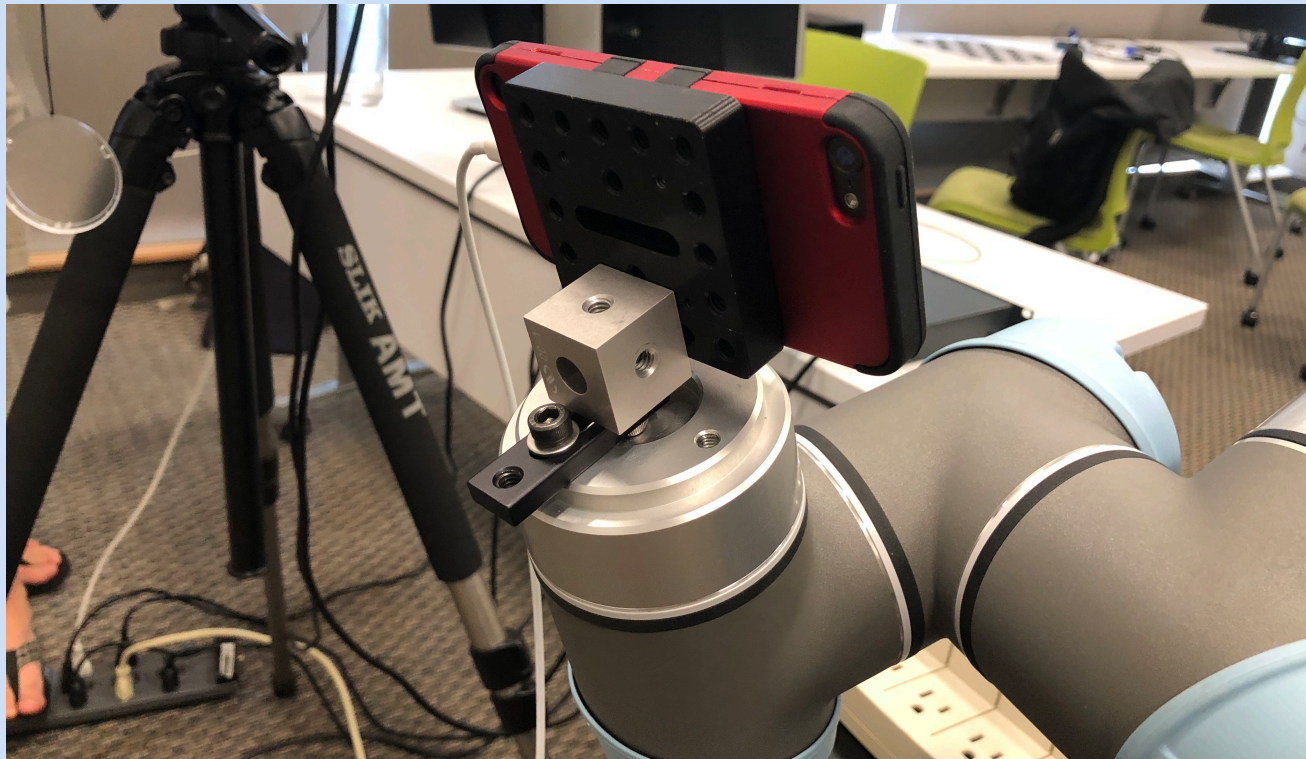
Fig. 5: Smartphone mounting to the tool head
