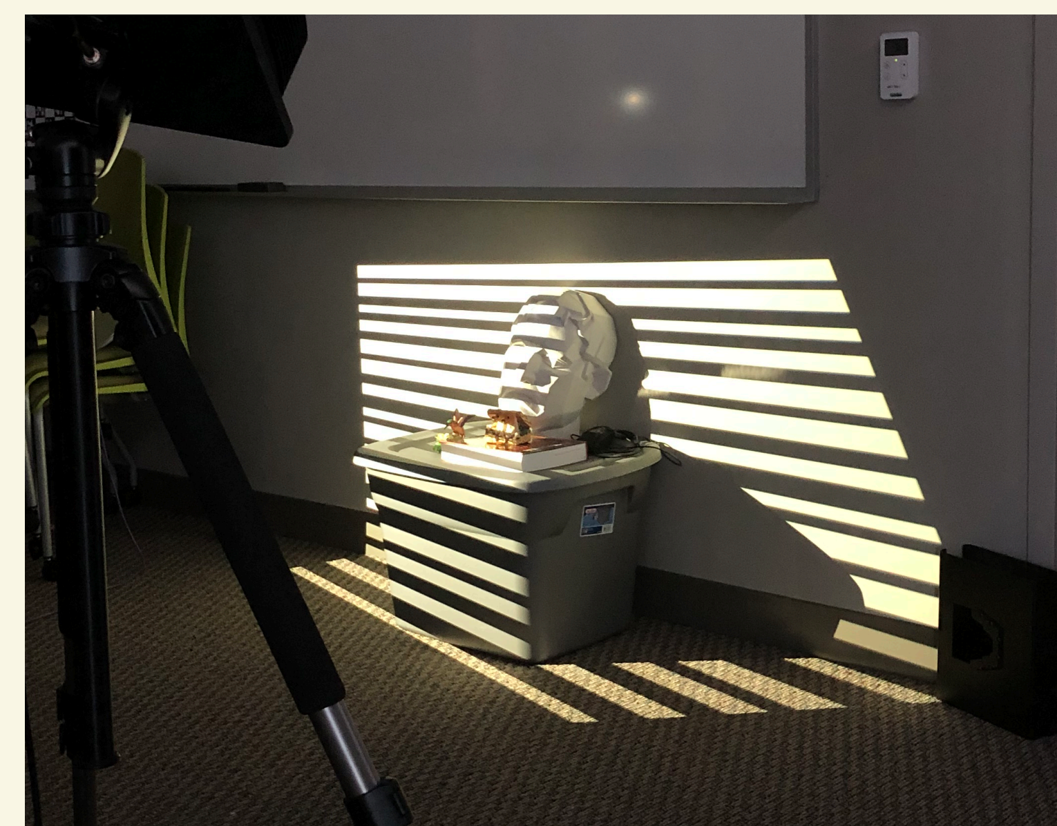
Fig. 3: projecting structured lighting onto a scene
