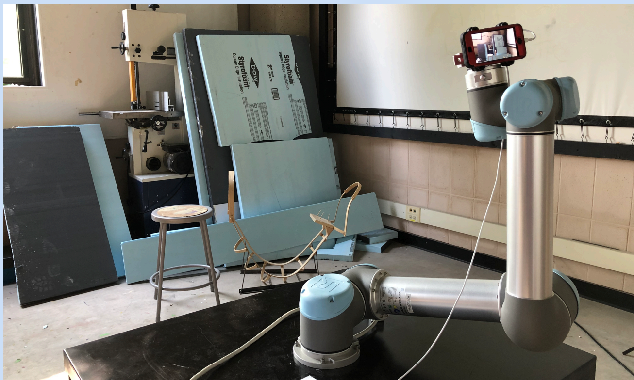
Fig. 6: Robot arm moving to different viewpoints during scene capture
